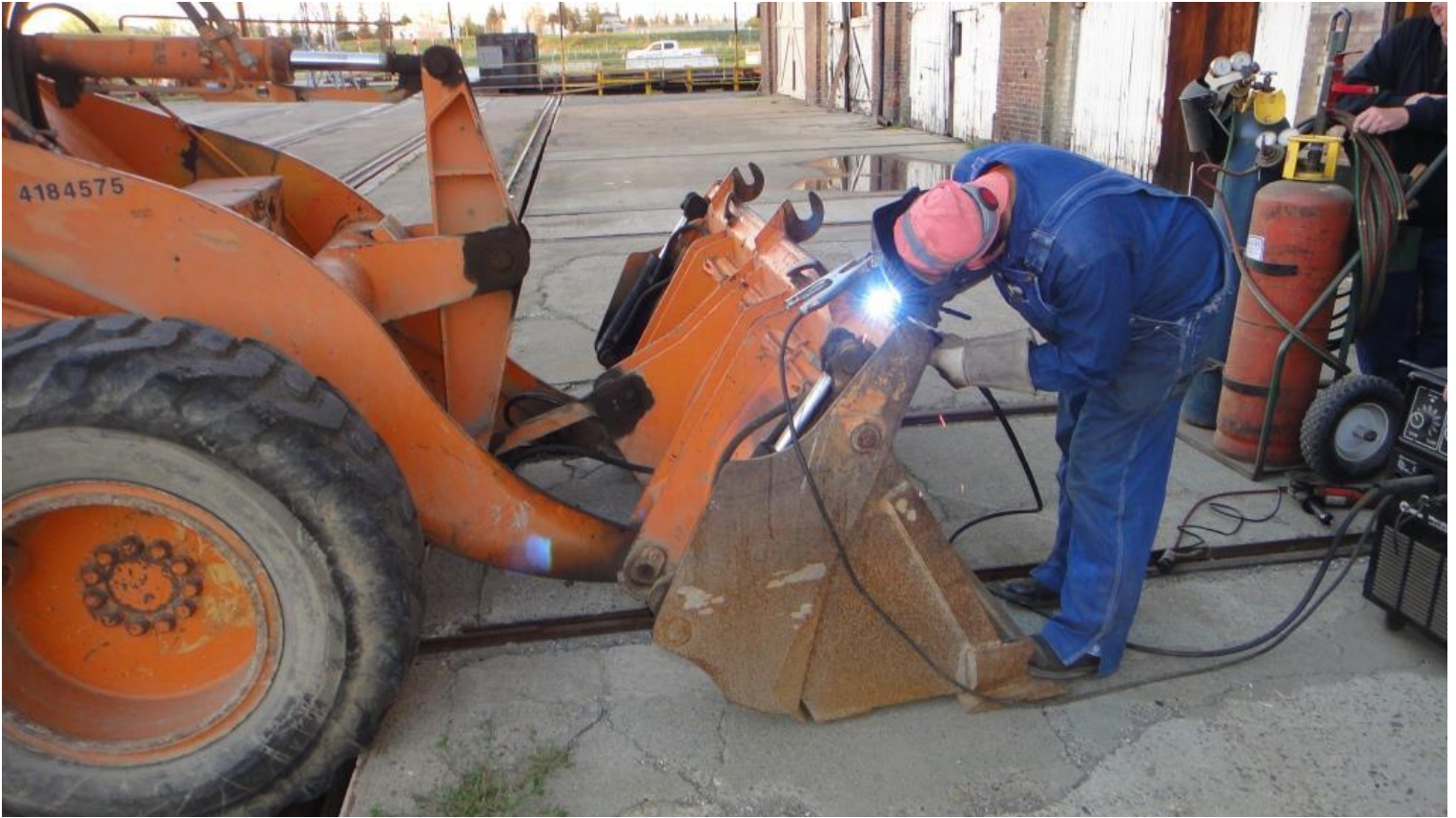
Then welds the crack
